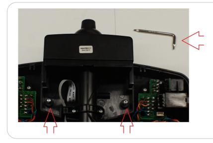
Using standard MPX hex screwdrive or any better screwdrive, remove two hex screws from your TX. After this deattach flex wire from the TX main board and remove comlete LCD mounting plastic case with LCD from the front panel.
