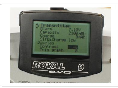
Now you can attach your battery back and try to power on your TX. From the contrast menu you can power ON and power OFF your TX LED backlight. If "Contrast" is "-6" or lower - backlight is turned OFF
