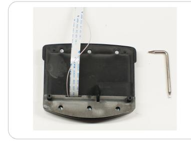
Check that you can assemble LCD mounting case without applying any force and than do it. Place each screw on it's place. And place LCD mounting case on it's place too. Than don't forget to mount it using two hex screw.
