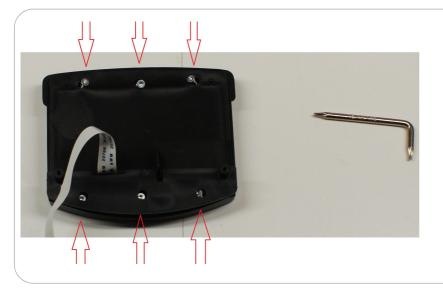
Remove 6 hex screws from the back of LCD mounting case
