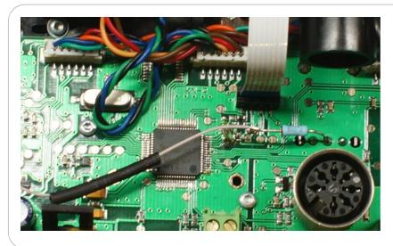
You need to solder the supplied 100R resistor between the teflon wire and middle pin of TX main switch. It's very simple, please don't forget to attach insulation tube.
